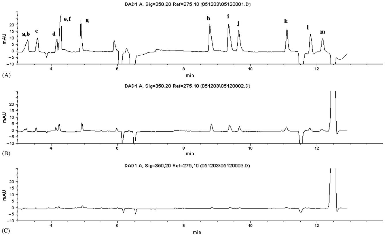
FIG. 2—Capillary zone electrophoresis separation of standard mixture of inorganic and organic anions, and carbohydrates at (A) original dilution, (B) diluted 1/5 with water, and (C) diluted 1/25 with water. Experimental conditions are described in capillary electrophoresis analysis section. See Fig. 1 for compound identity and concentration of original dilution.
