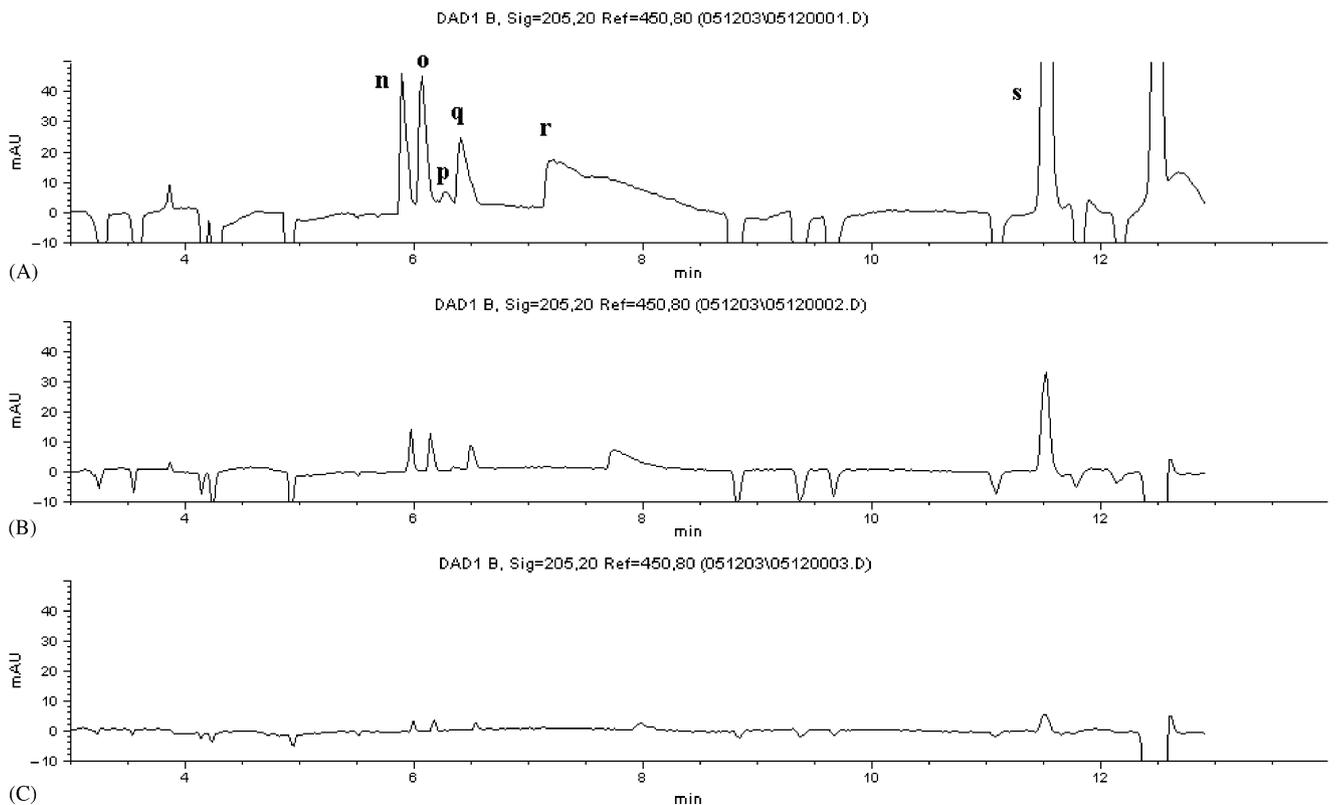
FIG. 3—Capillary zone electrophoresis separation of standard mixture of acidic adulterants at (A) original dilution, (B) diluted 1/5 with water, and (C) diluted 1/25 with water. Experimental conditions are described in capillary electrophoresis analysis section. See Fig. 1 for compound identity and concentration of original dilution.
