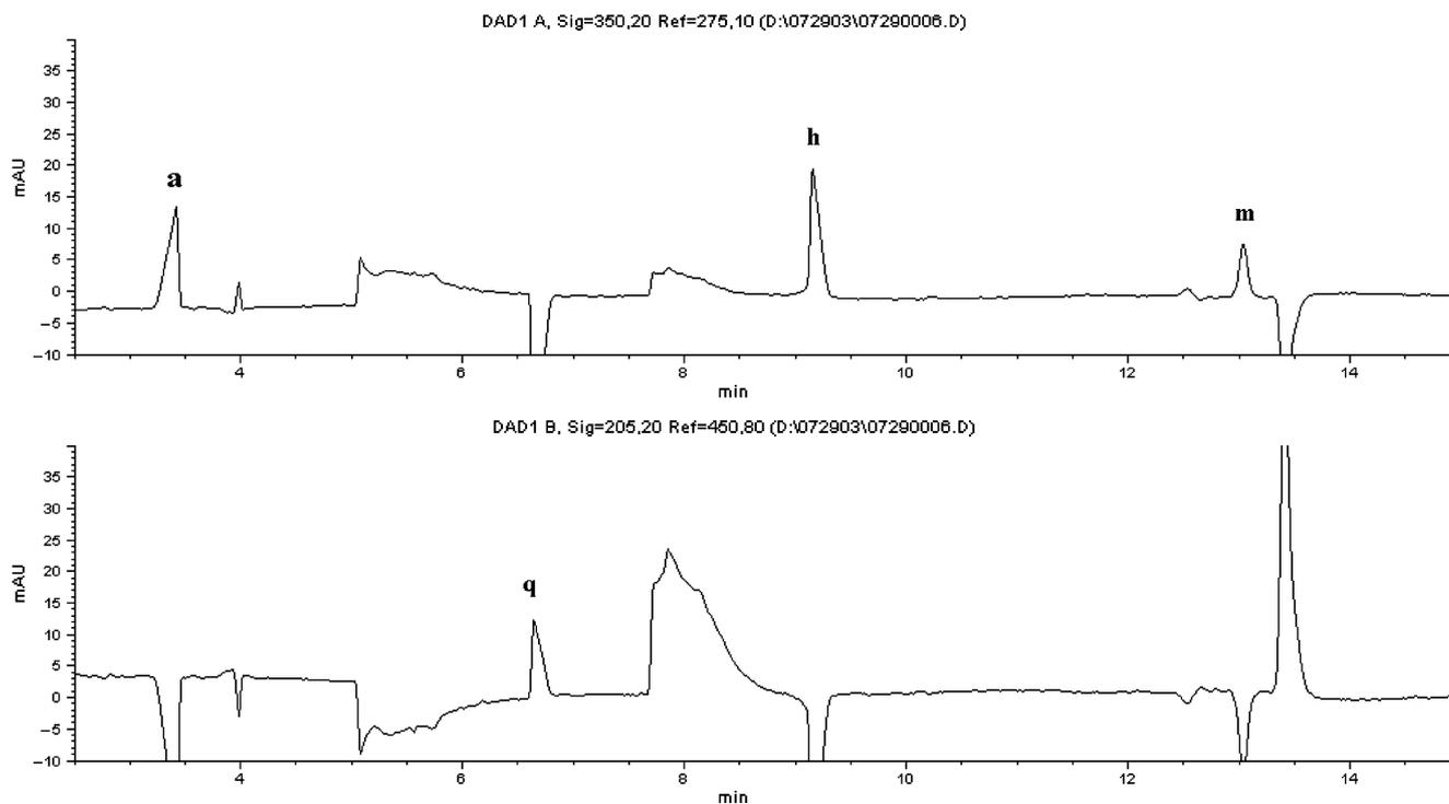
FIG. 4—Capillary zone electrophoresis of a seized heroin sample. Experimental conditions are described in capillary electrophoresis analysis section. See Fig. 1 for compound identity.
